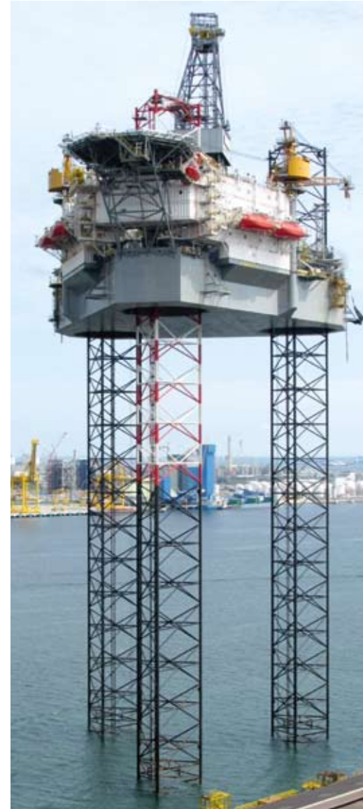
Discovery Triumph, the world's first KFELS Super A Class rig, is a robust and cost-effective drilling rig for harsh environments
